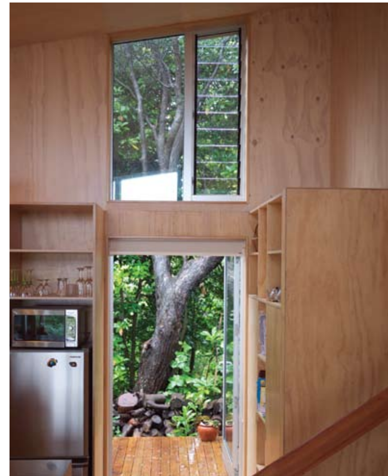
To keep waste and costs to a minimum, the interior of the house was built in natural pine plywood throughout, limewashed above 2.4 metres for effect. opposite page The building's footprint was shaped to incorporate the mature trees surrounding it, in order to connect with the existing natural environment.
